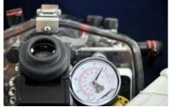
Stop pumping when the green LEDs light. Remove the input fitting from the vacuum connector.
