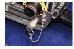
Once your camera is in place and the housing is closed, remove the block-off plug from the vacuum connector
