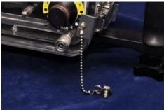
If salt water is left to evaporate, the salt will crystallize and could create a leak. To solve, soak the area in fresh water to dissolve the salt crystals. To prevent, thoroughly rinse your housing after every dive. If you cannot rinse it immediately following the dive, keep the housing covered/damp and then give it a good soaking once fresh water is available.
