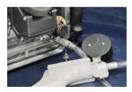
When the vacuum reaches about two inHG, the red LEDs will begin blinking at a fast rate.
