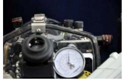
Insert the block-off plug into the vacuum connector. It is important to keep the blockoff plug in the vacuum connector whenever the pump is not connected.
