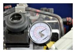
The flash rate of the red LEDs will slow when the vacuum reaches six inHG.
