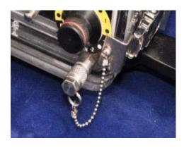
if exposed to enough pressure. With the plug installed, the vacuum connector can handle pressure of 4,000 psi. Our testing shows that the vacuum connector without the plug will leak when exposed to a pressure of 80 psi which is equivalent to 150' of depth.
